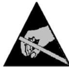
**Warning:** Failure to follow these instructions may result in damage to the unit due to electrostatic discharge. The electronic components of the humidifier control are very sensitive to electrostatic discharges. In order to safeguard these components during installation and servicing, steps must be taken to protect against ESD.
