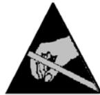
**Warning:** The electronic components of the humidifier control are very sensitive to electrostatic discharges. In order to protect these components during any type of installation, steps must be taken to guard against damage from electrostatic discharge (ESD protection).
