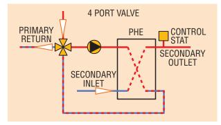
Typical Schematic for Unvented HT-Breeze/Buffer Application
